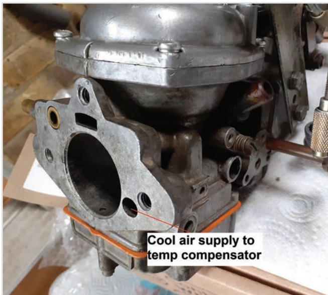
Pic 9. Air supply hole for temperature compensator
