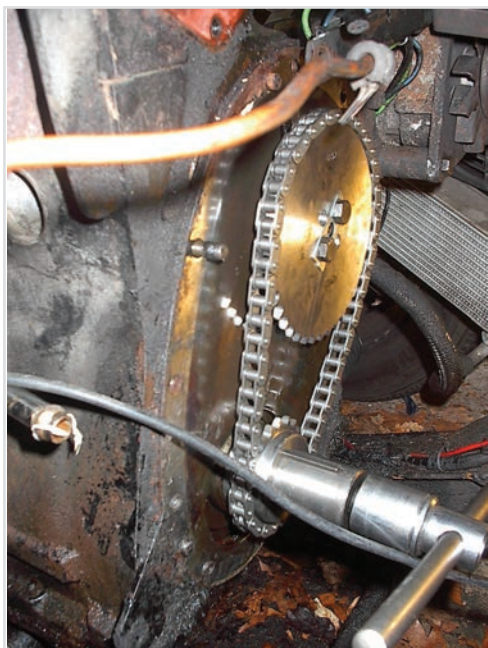
Timing Chain and Gears Replacement on my car
