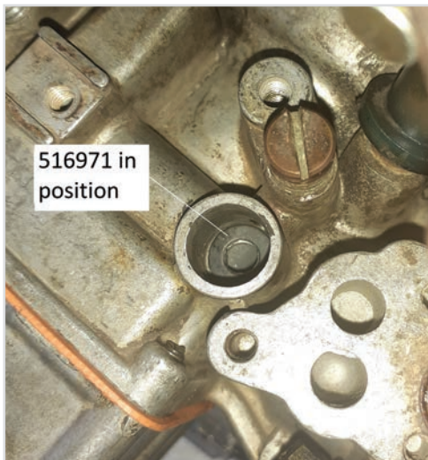
Pic 9. Insert smaller seal (516971) into carb body
