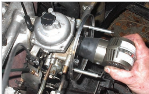
Balancing the Carbs on my car using a Webber Synchrometer for tuning them
