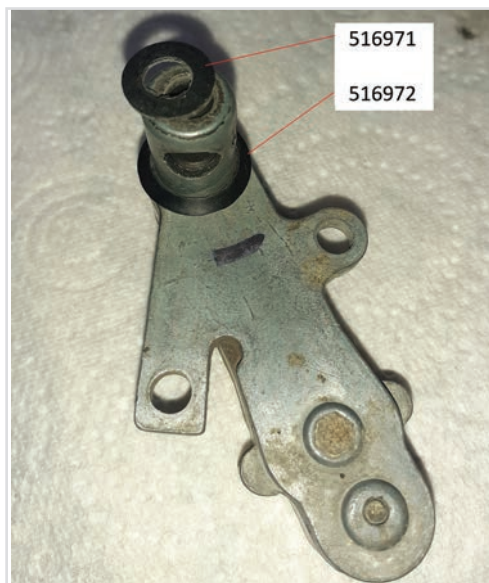
Pic 8. The two seal positions
